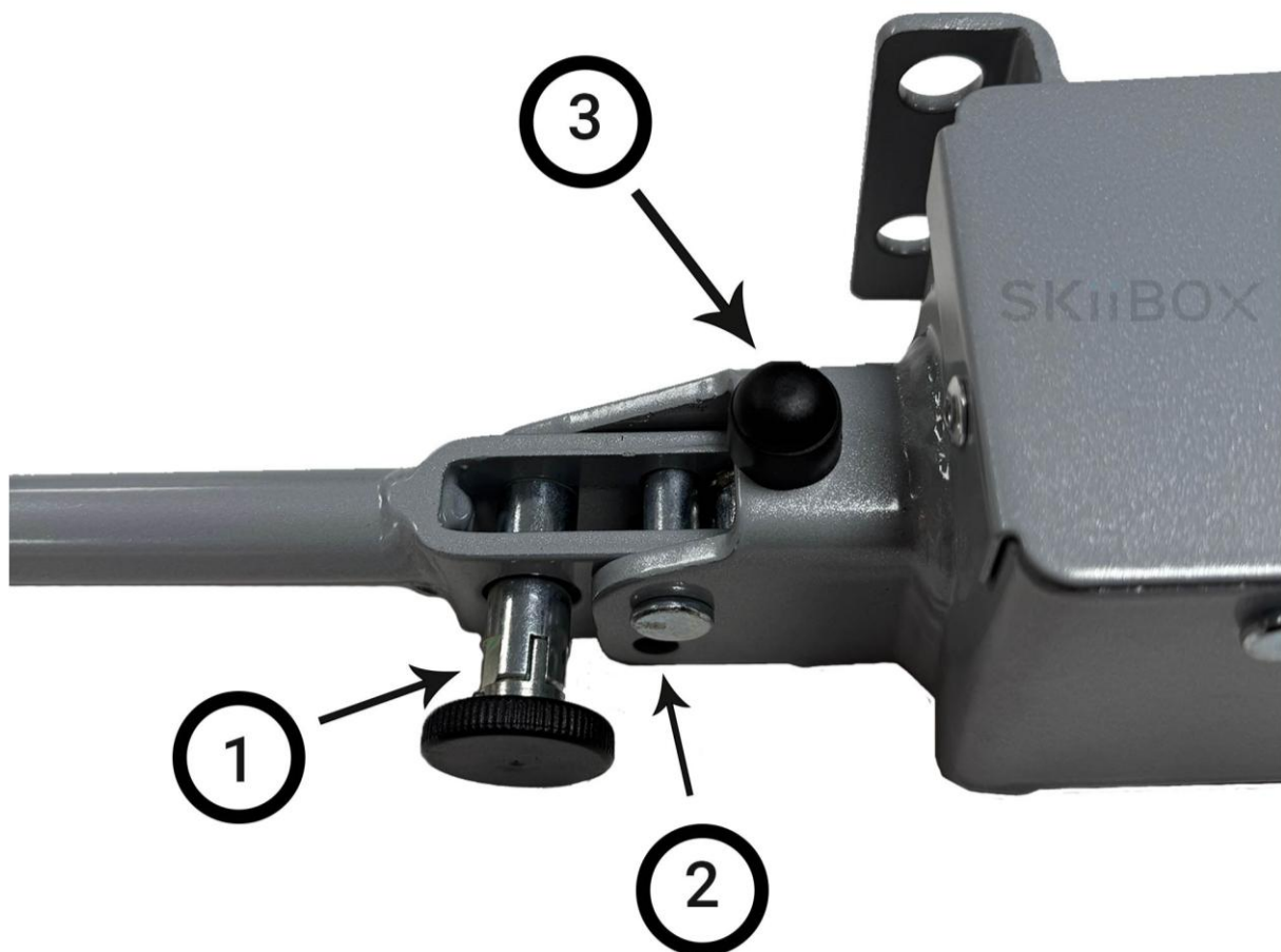
Figure 3: Close-up image of the safety bolt (1), the additional hole for a padlock (2) for theft protection, and the fixing screw (3). The fixing screw allows for adjustment of the safety bolt if it becomes misaligned.
